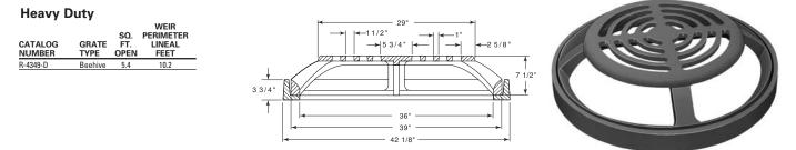
For use in narrow median on divided highways, freeways or expressways. Provides large capacity drainage when required during heavy rainfalls.
